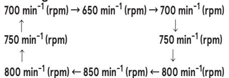
Buzzer makes one short sound when the engine speed is set to  $650 \text{ min}^{-1}$  (rpm), indicating the minimum trolling speed is set.
