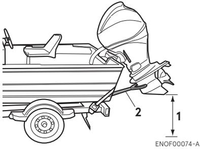
1. Ground clearance should be provided sufficiently.
