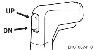
2. Pull the tilt stopper down as shown below drawing.
