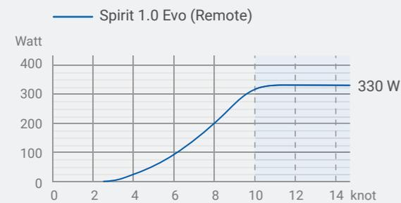
\*The hydrogeneration data is based on real tests with the anti-ventilation plate installed.
