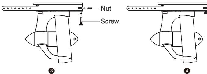
3. Drill on the rudder: Keep the rudder mounting hardware perpendicular to the rudder, select two holes as far as possible, and mark on the rudder. Then drill two  $\Phi 4.2$  holes.
