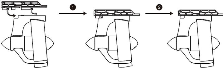
2. Attach the rudder mounting hardware onto the US fin box adapter: Insert rudder mounting hardware into the adapter, then fix it with a screw and a nut.
